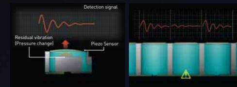
The piezo element [sensor] detects the residual vibration (pressure change) in the ink chamber and diagnoses the nozzle condition. If a clogged nozzle is indicated by an irregular vibration pattern, the printer automatically adjusts the print quality.
